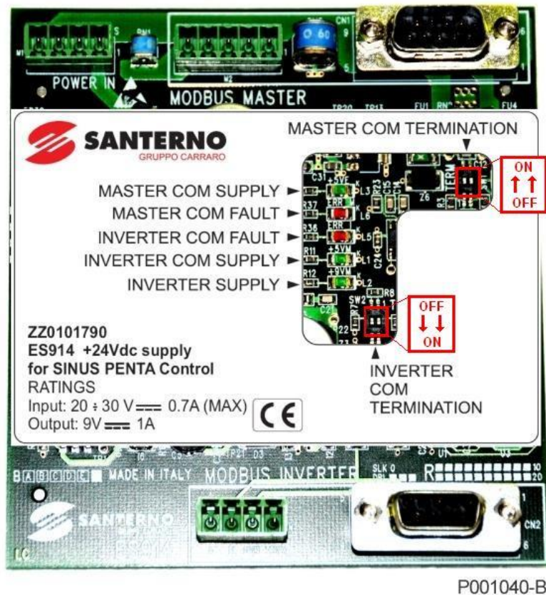
Figure 177: Position of the LEDs and DIP-switches in ES914 board
