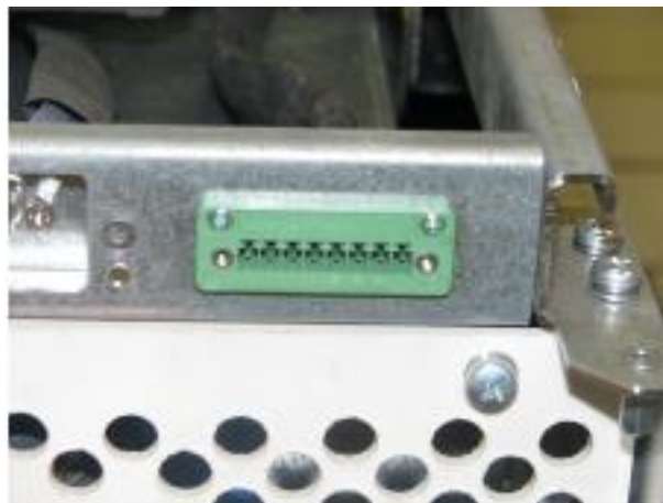
Figure 23: BRAKE connector supplied with the drive
