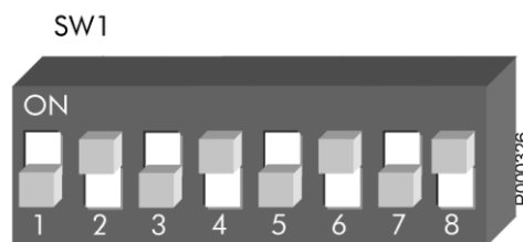
Figure 79: DIP-switch SW1 setting for five-channel mode
