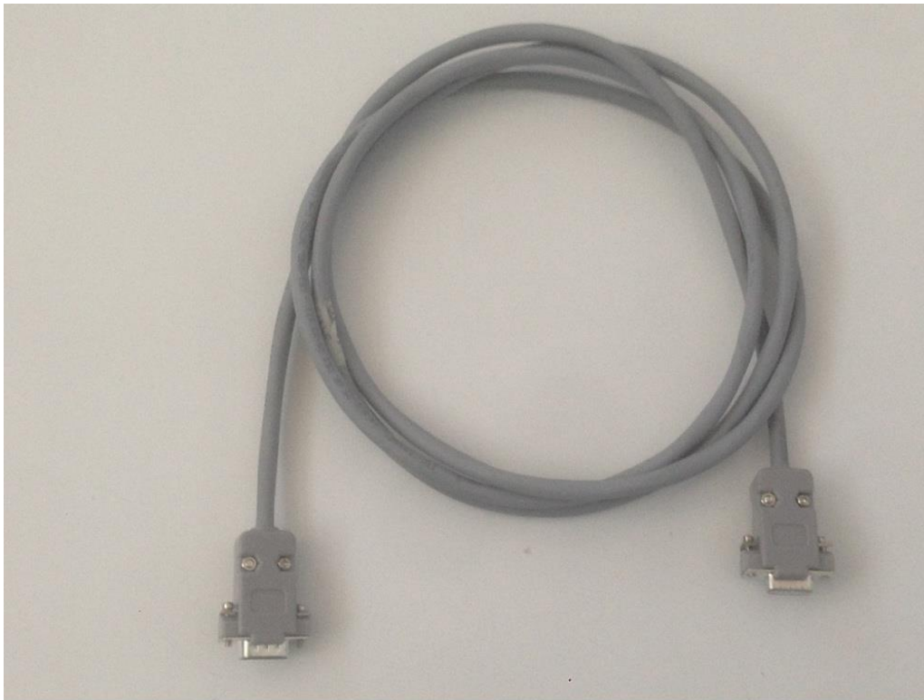
Figure 12: Example of a 9-pin shielded cable for signal connection
